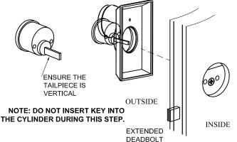
5. From the inside of the door orient the turn piece mounting plate and secure by inserting the two 2" pan head machine screws through the turn piece mounting plate, lock, and into the cylinder housing.
