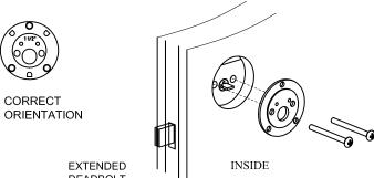
6. Install the Internal turn piece trim by positioning the turn piece THUMBTURN HORIZONTALLY over the mounting plate, inserting the cylinder tailpiece into the turn piece. Secure the turn piece in place by fastening two 1/2" turn piece mounting screws through the two countersunk holes on the turn piece.
