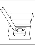
place using (2) combo screws. 10. Secure the latch strike in
