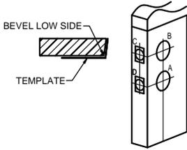
2. Determine the backset and mark the backset center points (A, B, C, D) on the template. The most common backset is 2-<sup>3</sup>/<sub>8</sub>".
