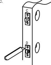
5. Chisel faceplate marking to a depth of <sup>1</sup>/<sub>8</sub>" or until faceplates are flush with door edge.
