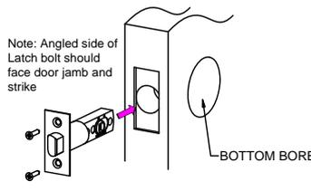
8. Deadbolt latch has been preset to 2-<sup>3</sup>/<sub>8</sub>" backset. If the door is prepped for a 2-<sup>3</sup>/<sub>8</sub>" backset No adjustment is required. Only for a 2-<sup>3</sup>/<sub>8</sub>" backset, adjust the deadbolt latch by rotating it counter clockwise until you reach the END of the turn to fit a 2-<sup>3</sup>/<sub>8</sub>" door prep.
