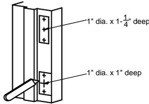
22. Chisel out the area marked in step 24 until the latch and deadbolt strike (with reinforcing if applicable) are flush with the door. The approximate latch and deadbolt strike (without reinforcing plate) depth should be  $\frac{1}{16}$ " deep. If using the reinforcing plate with the deadbolt strike the depth should be  $\frac{7}{32}$ ".
