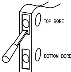
6. Latch is preset to 2-<sup>3</sup>/<sub>8</sub>" backset. Only for 2-<sup>3</sup>/<sub>8</sub>" backset, Adjust the latch bolt to the correct backset (typically 2-<sup>3</sup>/<sub>8</sub>" or 2-<sup>1</sup>/<sub>4</sub>".)
