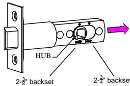
7. Insert the latch bolt into the bottom bore ensuring the curved side of the bolt is facing the door jamb. Using a <sup>3</sup>/<sub>16</sub>" drill bit, drill two pilot holes and secure the latch to the door using two combination screws. DO NOT OVER TIGHTEN COMBO SCREWS.
