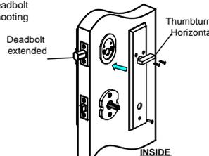
16. Plastic washers are already preinstalled on the levers. Place the plastic washer on the shank of the knob or lever. Spare washer is also packed
