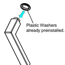
17. Press the lever snugly against the interior trim assembly and tighten the set screw with the provided Allen wrench. **Note:** The set screw should be located on the inside of the lever to engage into the spindle groove.
