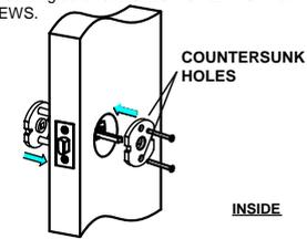
13. Install the External Backplate on outside of the door. Ensure to extend the deadbolt using a screwdriver and insert the Cylinder Tailpiece through the + slot of the deadbolt with the cylinder tailpiece in a vertical position.
