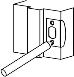
24. Secure the latch strike in place using (2) combo screws.
