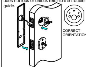
15. Position the interior trim over the mounting plate and insert the cylinder tailpiece into the thumbturn of the interior trim.
