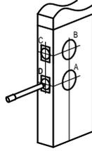
3. Carefully using a 2-<sup>3</sup>/<sub>8</sub>" diameter hole saw drill through holes A and B. Drill a 1" diameter hole through C and D. IMPORTANT: DRILL PERPENDICULAR (90°) TO DOOR.
