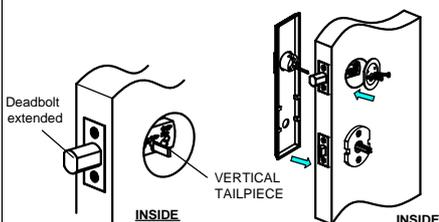
14. From the inside of the door orient the turn piece mounting plate and secure by inserting the two deadbolt mounting screws through the turn piece mounting plate, lock, and into the cylinder housing. Test the deadbolt by locking and unlocking the deadbolt with the key. If the deadbolt does not lock or unlock refer to the trouble shooting guide.
