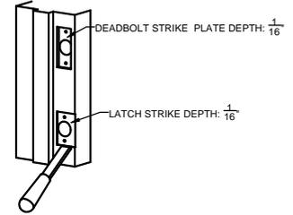
23. Using the latch strike plate as template mark and drill (2)  $\frac{1}{8}$ " pilot holes.
