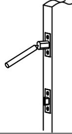
19. Align the center marking of the deadbolt with center marking of the deadbolt strike plate on the template. From the template mark, the mounting screw hole and center markings of the deadbolt and latch strike plate.
