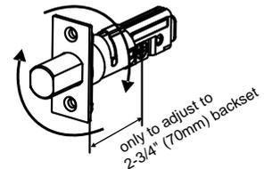
9. Insert the deadbolt latch into the top bore Ensuring the + Slot is underneath and ridge on top. Using a <sup>3</sup>/<sub>16</sub>" drill bit drill two pilot holes and secure the deadbolt to the door using two combination screws. If the deadbolt is not extended, insert a screw driver into the "+" slot and rotate counter-clockwise.
