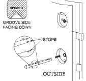
outside mounting plate over the spindle and insert the two legs of the mounting plate into the lock.
