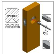
D. Install the inside adapter. Insert the two legs of the adapter into the holes in the latch support. Note: The inside adapter has countersunk screw mounting
