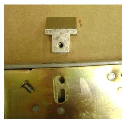
10.0 Reinsert Middle Latch Insert 10.1 Reinsert the latch insert into lock assembly.
